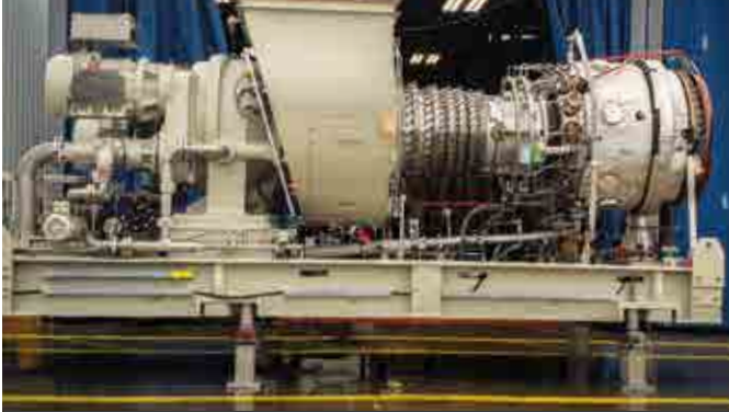
Left: One of the 15mw Solar Turbine Units. Right: 45 mw plant under construction.
